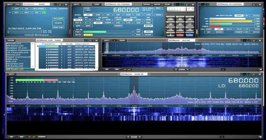
**SDR Uno – ExtIO Version** is the flagship program for the SDRPlay RSP series of radios. It's a little more challenging to set up than the others. You need to use the ExtIO version of SDR Play for the RTL-SDR dongle to work. https://www.sdrplay.com/you-can-use-sdruno-with-an-rtl-sdr-dongle-new-video-guide/
