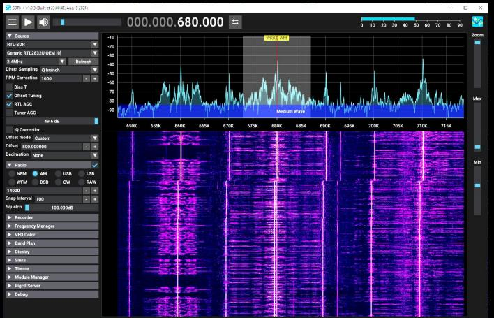
SDR++ https://github.com/AlexandreRouma/SDRPlusPlus currently available for Windows and Linux. Version 1.0 released: https://www.rtl-sdr.com/sdr-version-1-0-0-released/ Multi VFO, Wide hardware support, Full waterfall update, FM Stereo, Freq. Presets and more. Perhaps a little difficult for first time SDR users to operate.
